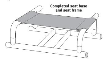
Locate the seat base and find the curved legs. With the curved legs to the front, insert the seat platform rails onto the pontoon frame posts.
